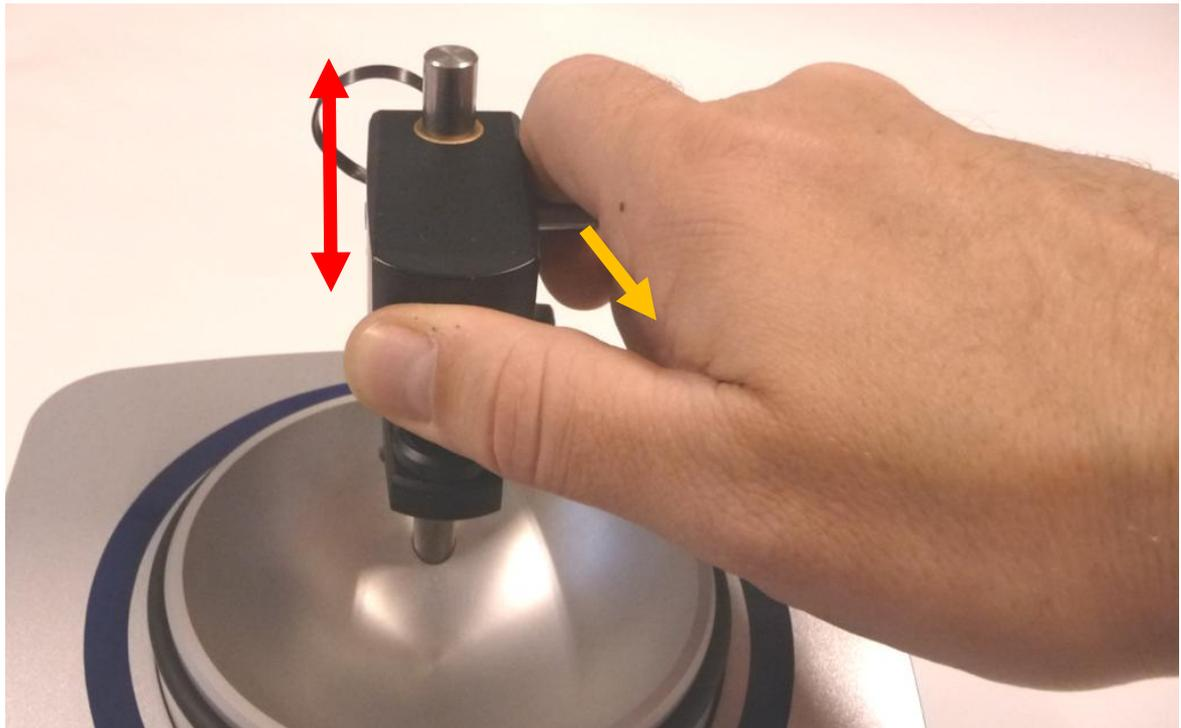
If the watch does not fit correctly into the space, you can also move the watch support vertically by loosening the screw on the side.
